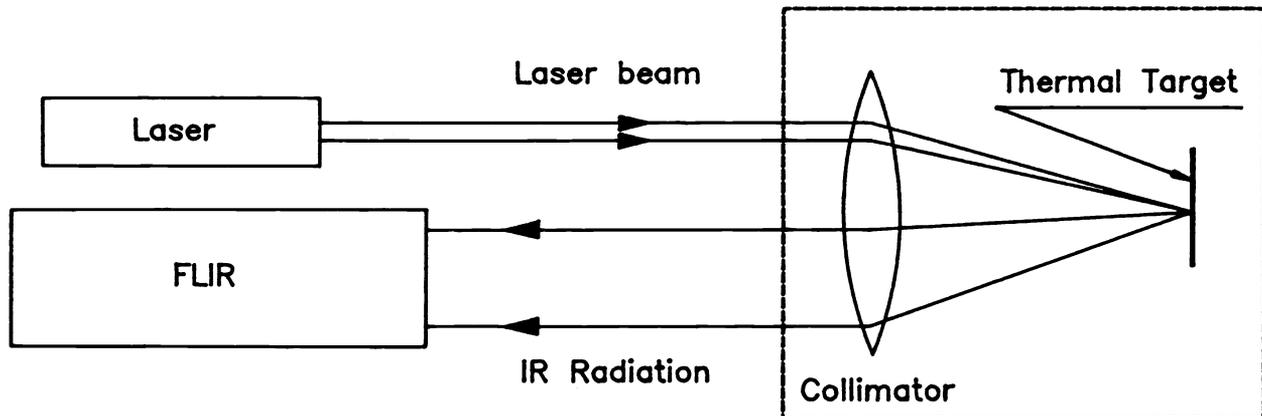
Figure 1. Schematic diagram of boresighting using the TT method.
