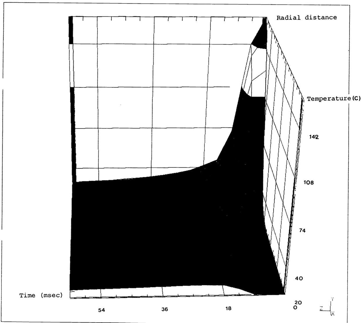
Figure 6. Thermal profile dependence on time and radial distance from heat spot center given by Finite Element Analysis.
