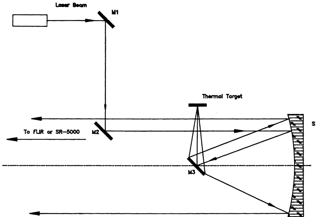
Figure 3. Thermal Target and optics set-up.
