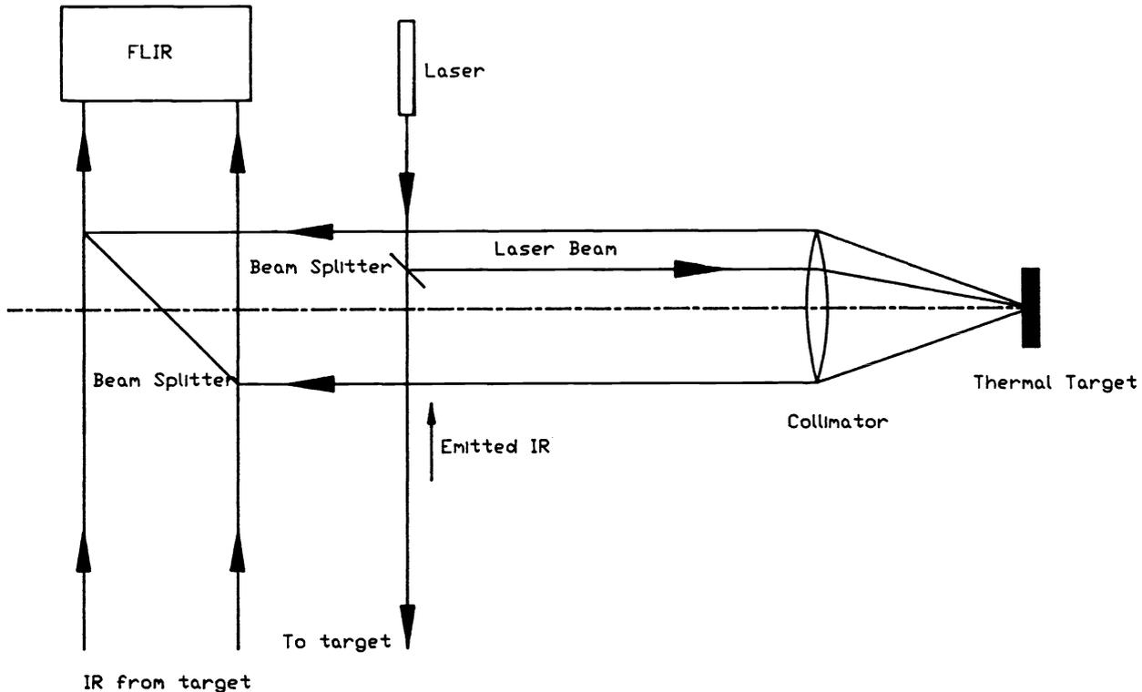
Figure 7. Schematic diagram of the real time boresighting using the TT method.
