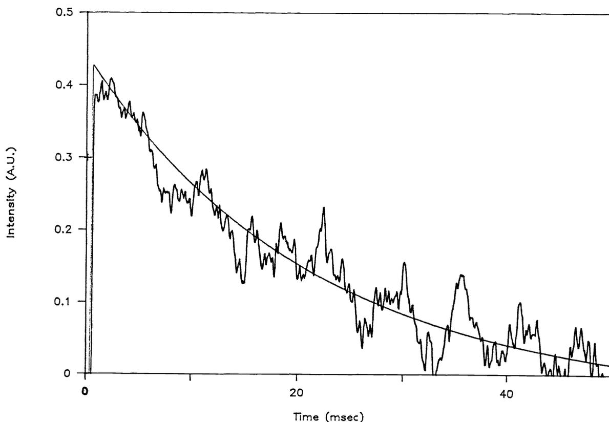
Figure 5. Time dependence of radiometer signal intensity from a single laser pulse on TT. The continuous curve is an exponential.
